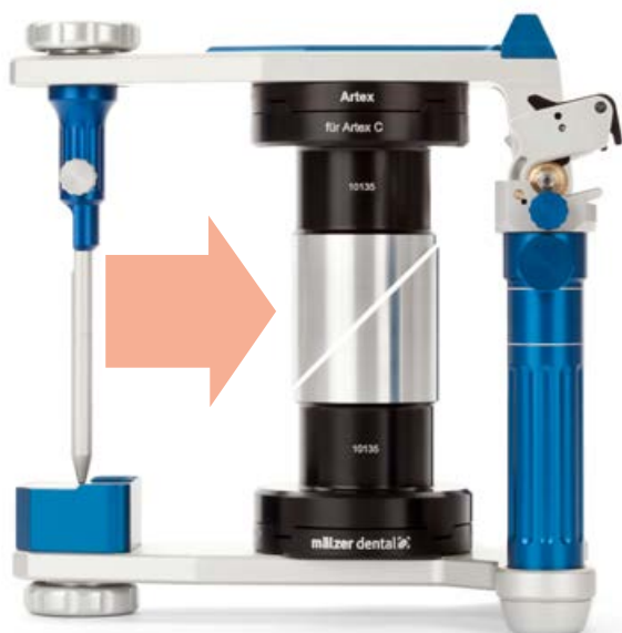
Articulator incorrect: clearly visible gap
