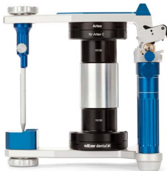
Properly calibrated articulator: gap-free closure
